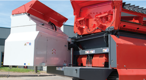
Hydraulically opening powerpack for ease of maintenance
