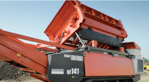
Tipping function activated by radio remote control
