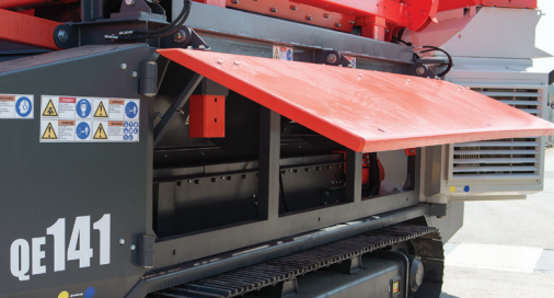
Hydraulically folding doors for easy access
